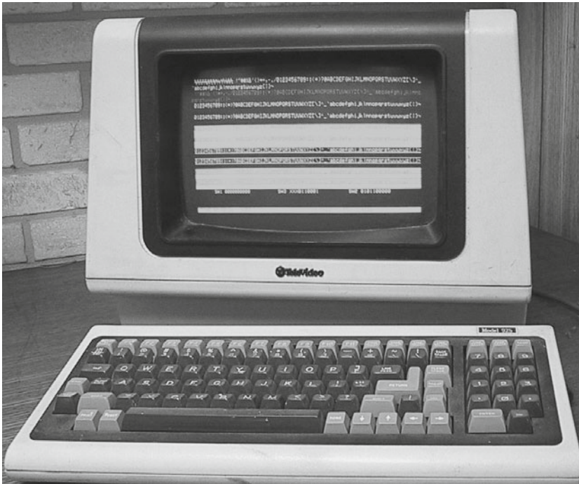
Figure 3-1. TeleVideo 925 computer terminal
