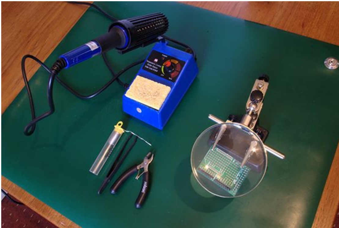
Figure 12-9: An example soldering work area, with a protective anti-static workmat
