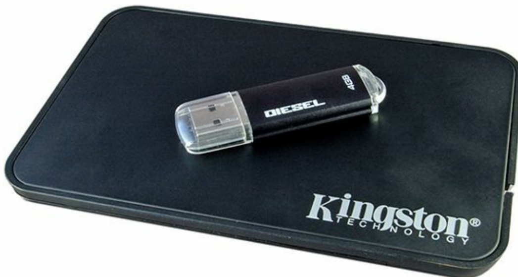
Figure 1-6: Two USB Mass Storage devices: a pen drive and an external hard drive
