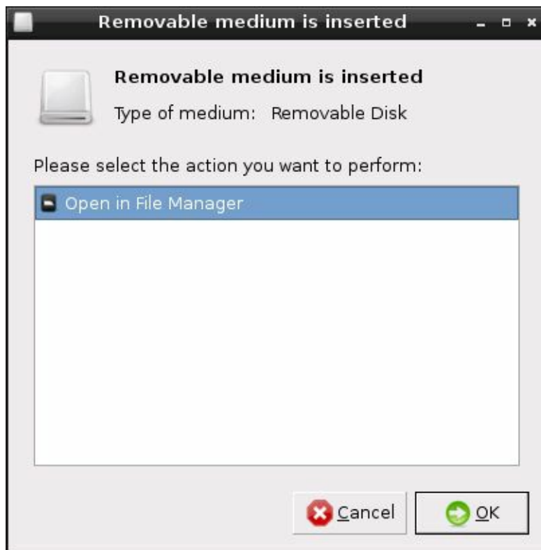
Figure 2-2: LXDE automatically mounting a USB mass storage device
