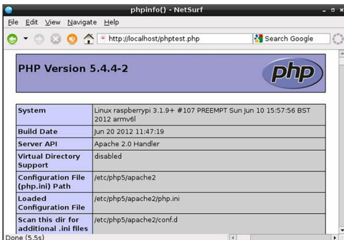
Figure 9-4: Testing Apache’s PHP module on the Raspberry Pi
